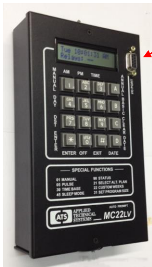
DB9 female connector for RS232 I/O
