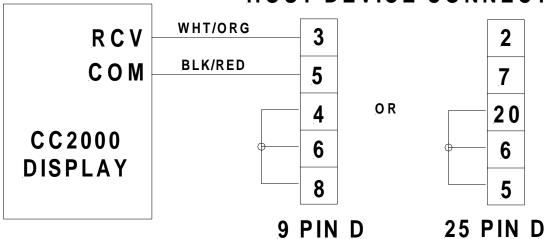
2400 BAUD, NO PARITY, 8 DATA BITS, 1 STOP BIT
