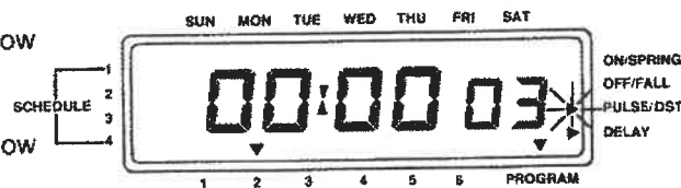
Figure 9 LCD Display After Selecting PULSE Event in DELAY Event Programming
