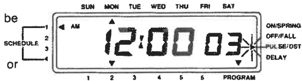
Figure 13 LCD Display After Selecting PULSE Event in TIMED Event Programming
