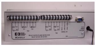
Be sure to follow all local wiring codes and to replace the TB cover after all wiring is complete.
