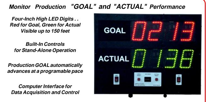
The AE44-503J provides: a programmable pace that automatically paces the "GOAL" display, a "COUNT" input that increments the count by one each time the input is activated, a "RUN/HOLD" switch to hold the pace during breaks or down periods, and separate "RESET" buttons for both the "GOAL" and "ACTUAL" displays. Painted Steel Enclosure (24"W x 18"H x 4"D).
