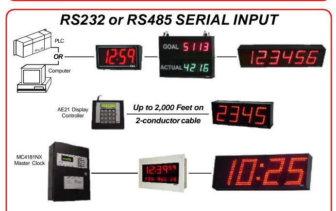
Send time or data to multiple displays throughout your facility. Ideal for computer or master clock controlled clock systems, timers, process indicators, and production monitors.
