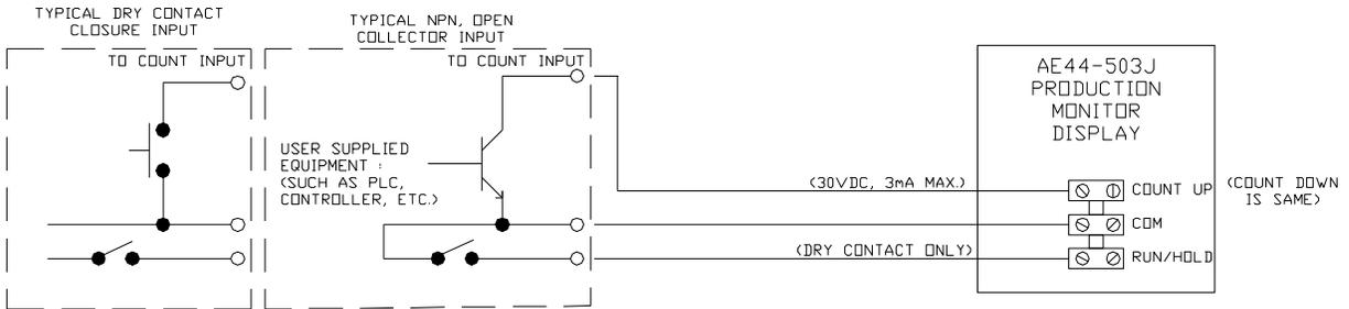
**TYPICAL WIRING EXAMPLES : COUNT AND RUN/HOLD INPUTS**
