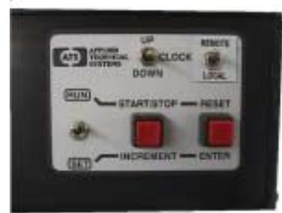
Typical built-in controls on the top panel. With the LOCAL/REMOTE in the LOCAL position, the AERFTX2 is locked out and will not control the timer. Set it to the REMOTE position for RF wireless control.
